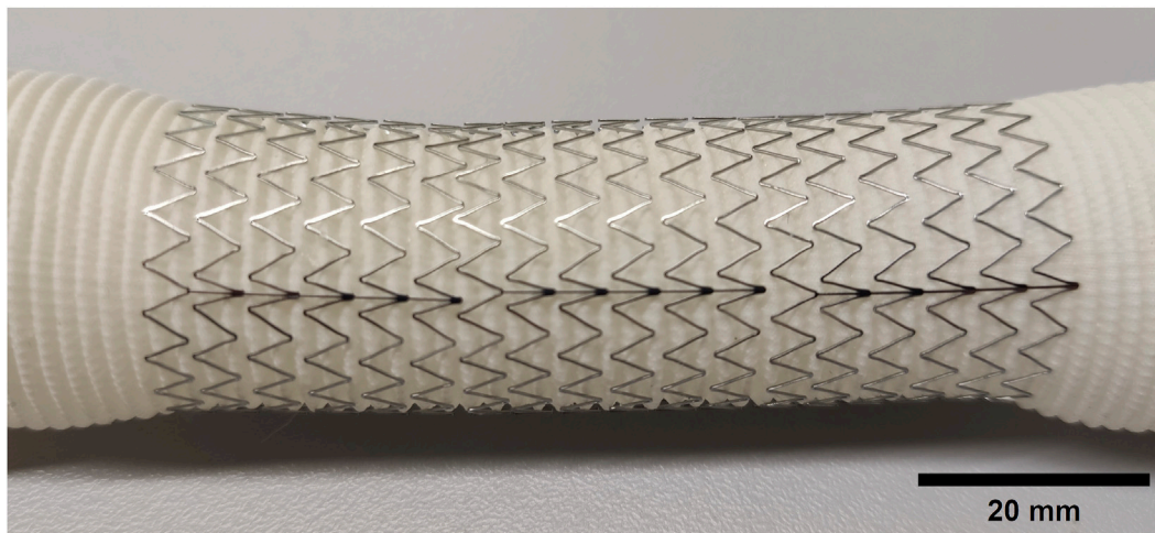
FIGURE 1 Photograph of a compliance-matching aortic graft.
